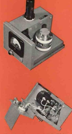
The oscillator unit can be disassembled quickly by removing the case scretcs. Wiring of frequency determining circuits is short and rigid.
